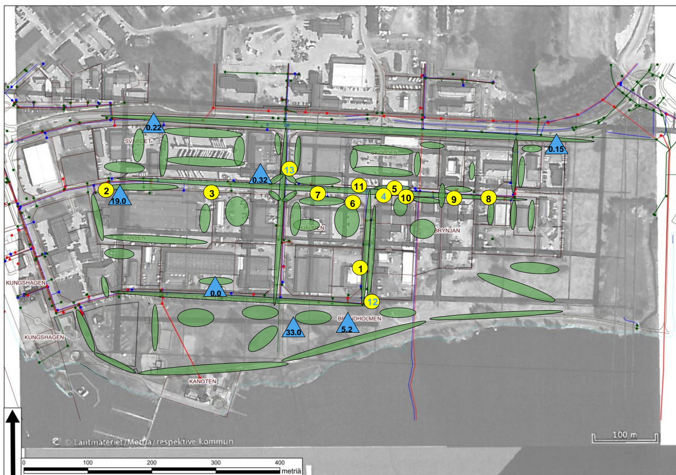
Figure 1. Mapped walk-over-survey areas. Green areas were surveyed with no sign of emission; yellow dots with black numbers indicate a response in analyser (0,2 ppm) and yellow dots with blue numbers indicate slightly more elevated TOC concentrations (0,3 ppm). Blue triangles are the groundwater sampling pipes; the numbers show TOC concentration of the gas (in ppm) in the head-space of the groundwater pipe.
